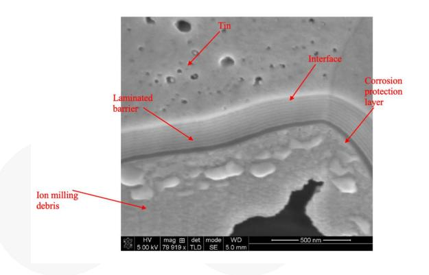
**Fig. 1:** FIB-cut SEM image shows the layer structure of a CCA (circuit card assembly) coated with250 nm ALD-Cap.
