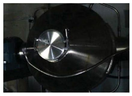
Forge Nana's LITHOS Rotary Blender Reactor System combines industry expertise in rotary particle handling with a deep understanding of ALD, resulting in an easy-to-use, flexible, and reliable production system. Forge Nana's system is designed to coat each particle with unrivaled thickness and conformity control, while minimizing or eliminating particle agglomeration. Our production machines are customizable and built to order, ensuring the optimal solution for each customer.
